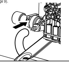
Install the handle and spray wand storage bracket
