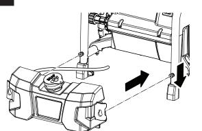
3 Connect injection hose to fitting on pump (see
