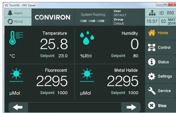
Figure 2-18 Virtual Chamber Displays
