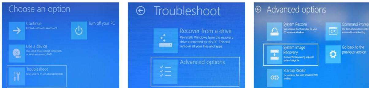
**Figure 7-37 System Image Recovery Sequence, CM v8.5 and Dell-Windows 10 Hardware**
