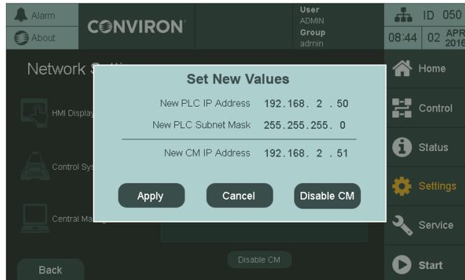
**Figure 2-12** CMP6060 PLC and CM Network Settings
