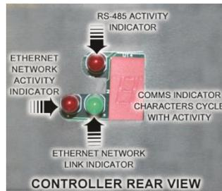
Figure 7-24 CMP5090 Indicator LEDs
