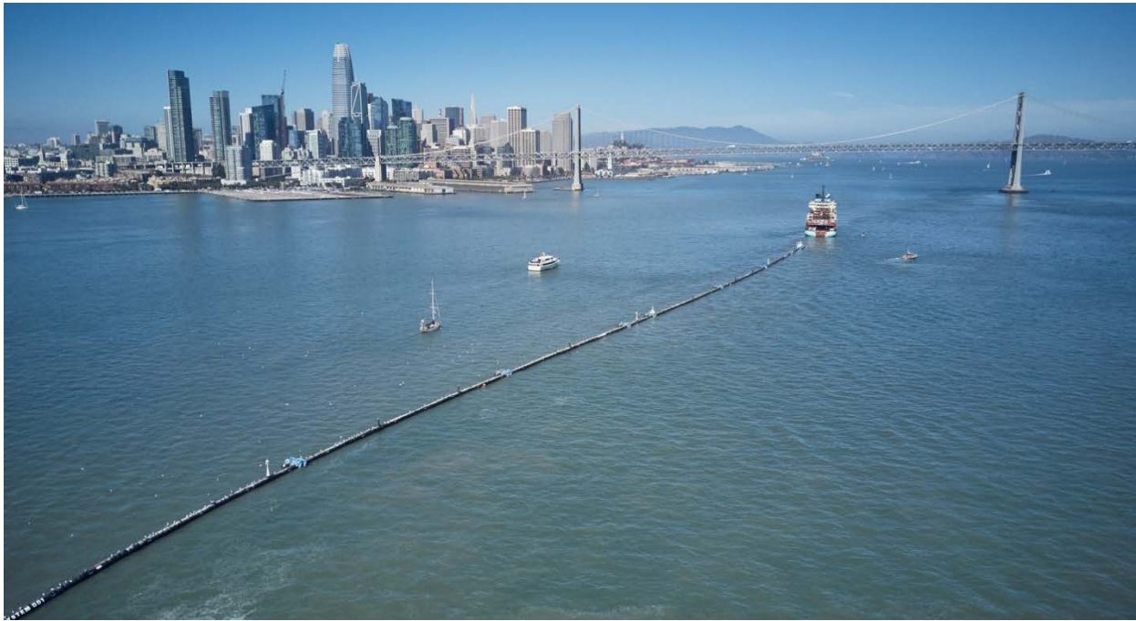
Figure 1 The Ocean Cleanup Foundation system using a floating boom to concentrate marine debris for removal from our oceans, measuring at length of 600m with a skirt underneath that prevents marine debris from escaping the system. Adapted from The Ocean Cleanup Foundation. Copyright [2018]. https://www.theoceancleanup.com/media-gallery/
