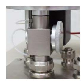
carousel to add samples it is only necessary to turn the valve, isolating the entire carousel section. The carrier gas will continue to flow through the rest of the analytical circuit. After adding samples to the carousel, close the lid, turn on the purge flow and let the carousel purge for 2-5 minutes. Close the purge vent, turn off the purge flow, and open the isolation valve.
